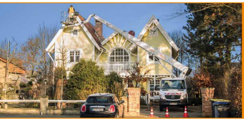
**RUTHMANN** STEIGER®® **TBR 250** The new 25 m class on a 3.5 t truck
