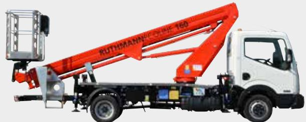
The most **compact ECOLINE** model in the series scores with its optimum working height, lateral outreach, and curb weight. It is also **very easy to handle**, making it ideal for **municipal/inner-city** assignments and the vehicle of choice for **equipment rental companies**.
